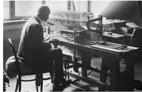
Machine for punching Jacquard-cards, Munichs Silk-Art Weaving Manufacture Gerdeisen, about 1920, Foto: Deutsches Museum, Munich
